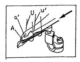
WHEN MOVABLE KNIFE (A) RETREAT FROM ITS LEFTEST DEAD POINT TO THE RIGHT, HOOK BLADE (8) AND (8') WILL PULL THE NEEDLE THREAD AND LOOPER THREAD TO THE FIXED KNIFE AND. CUT THE THREADS IN ORDER AND THE CLAMP SPRING WILL HOLD THE THREAD END AND MOVE TO THE BACK OF LOOPER TOGETHER WITH TRIMMING KNIFE SET (A). YOU CAN ADJUST THE HOLDING PRESSURE OF CLAMP SPRING TO AVOID THE THREAD END CAME OFF DURING THE MOVEMENT BY ADJUST CLAMP SPRING PRESSURE ADJUSTING PIECE.
